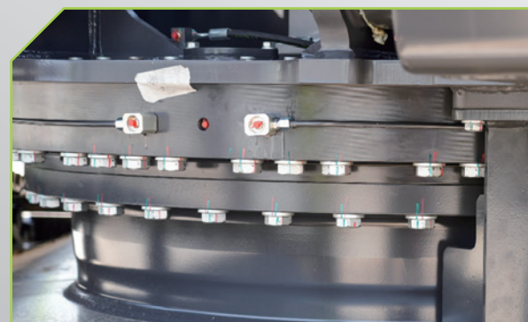
Add the centralized lubrication function of the swing bearing, to make the maintenance more convenient. 增加回转支承的集中润滑功能,保养更方便。
