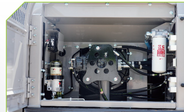
The inspection and maintenance of the oil filter, diesel filter and pilot filter are easily accessible at ground level, realizing one-stop maintenance. 机油滤、柴油滤、先导滤的检视与保养均伸手可及,实现一站式保养。
